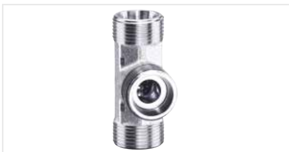
WV - Alternating valve: These valves permit the passage of flow from either inlet 1 or 2 to the outlet port whilst shutting of the inlet port not in use. The shutting off, of an inlet is achieved by a floating ball bearing which moves by the pressure of the flow.
